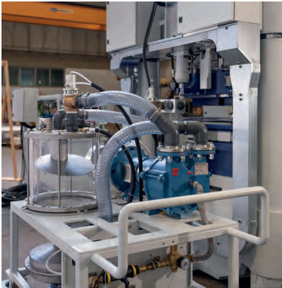
Water suction system „Wave“ for the manufacture of single layer tiles Difference between double and single layer tiles
