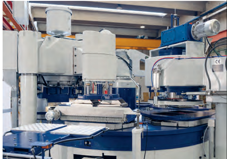
Automatic fresh tiles extracting shovel SLIM240 and its cleaning rotating brush
