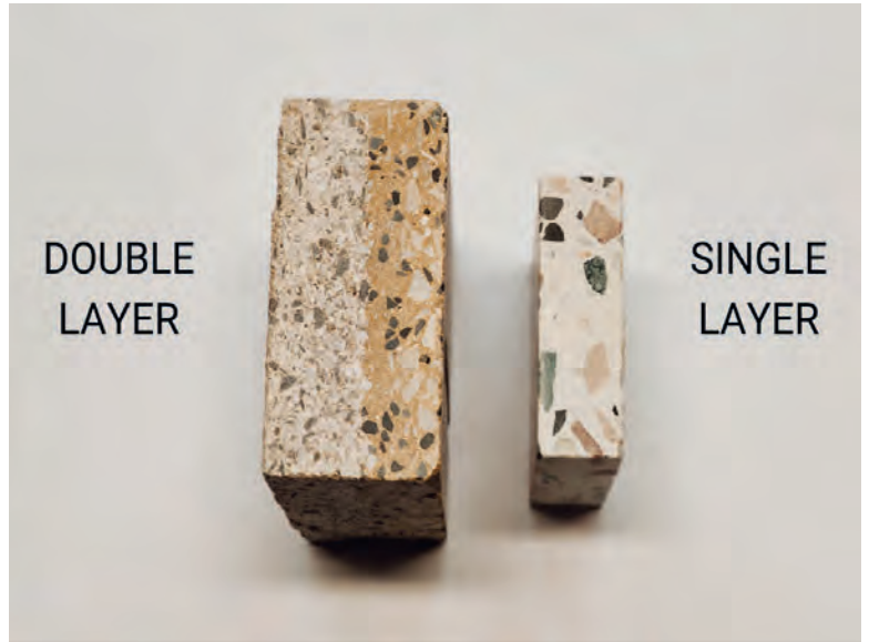
Water suction system „Wave“ for the manufacture of single layer tiles Difference between double and single layer tiles
