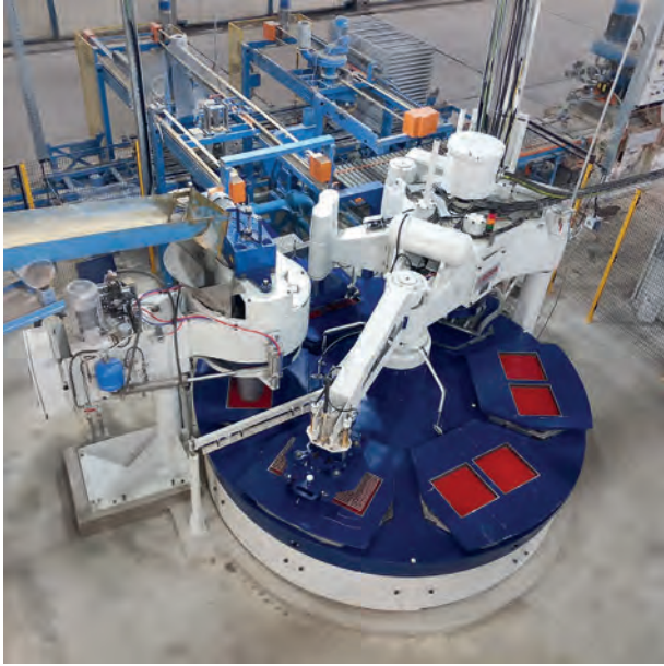
OPA740/6 equipped to man- ufacture single layer tiles
